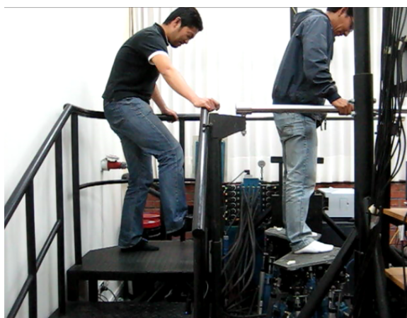
Figure 10. Tele-rehabilitation platform for gait training: Guidance control mode.
