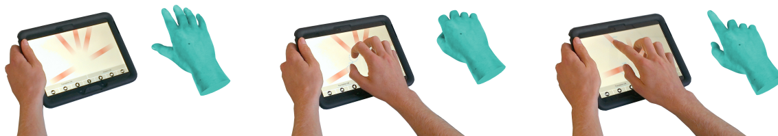
Figure 2. THING enables the control of 3D hand models (in blue) by sliding fingers along sliders arranged in a morphologically-consistent pattern on the tablet's screen. This creates a strong correspondence between user's input and pose of the controlled hand. Here, the user closes the virtual hand and then points the index finger.
