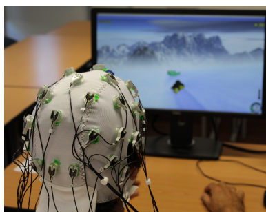
Figure 17. A subject using motor imagery, i.e., imagining left or right hand movements to manipulate Tux to catch fish.
