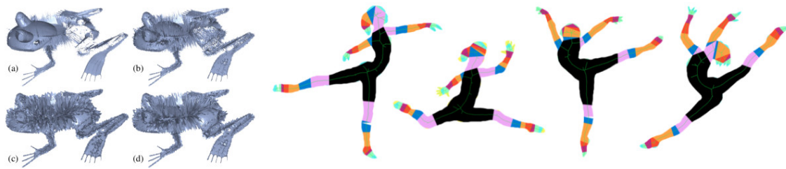
Figure 3. Left: Illustration of comparative study of 3D medial axis quality in [21]. Right: Hierarchies for similar shapes (dancers) in different poses to show that the proposed hierarchy is stable under articulation [22]. Coarser levels of the hierarchy are consistent even if finer levels are added in the presence of finer details. Also, note that the hierarchy is retained even with occlusion: The pink level of the left arm of the first dancer is occluded, but the blue level begins as it should.
