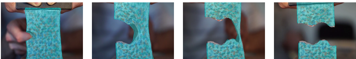
Figure 5. An augmented elastic object is torn. The cut is detected and applied to the virtual model in real time.
