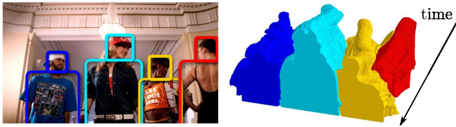
Figure 12. Results of our method applied to multi-person segmentation in a sample video from our database. Given an input video together with the tracks of object bounding boxes (left), our method finds pixel-wise segmentation for each object instance across video frames (right).
