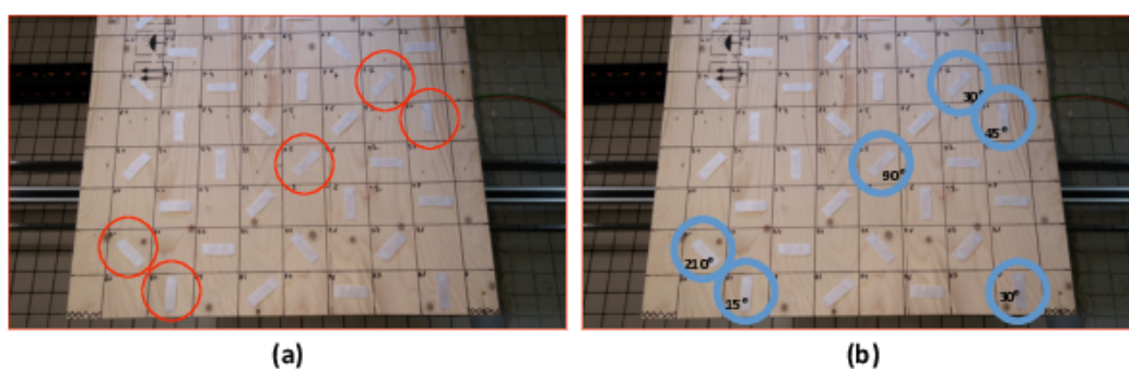
Figure 4. (a) initial read, 20% of the tags are missing (b) After 210 deg of rotation, all the tags are recovered
