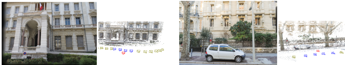
Figure 3. Image-Based Rendering (IBR) techniques use input photographs and approximate 3D to produce new synthetic views.
