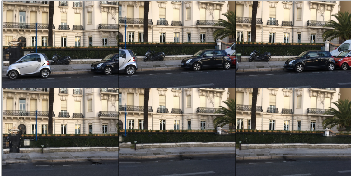
Figure 11. Our system takes as input a set of images from the same scene (top row). The method then removes all the vehicles in a multi-view coherent way (bottom row).
