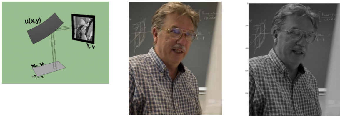
Figure 10. A constant source to a prescribed image (center). The reflector is computed (but not shown) and a resimulation using ray tracing shows the image reflected by the computed reflector.
