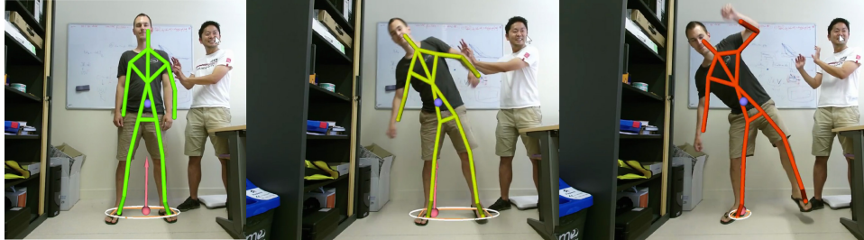
Figure 6. PersoBalance: Online stability estimation, from left to right: as a subject undergoes an unexpected external push, the system automatically estimates the ground reaction forces (pink arrow) and computes a stability index from the position of the ZRAM point relative to the support polygon (white/orange). The skeleton colour changes from green to red as the stability index decreases.
