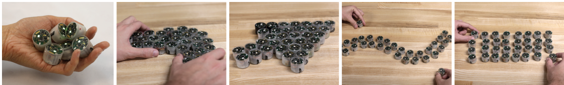
Figure 3. Zooids can be held as tokens, manipulated collectively or individually, behave as physical pixels, act as handles and controllers, and can move dynamically under machine control. They are building blocks for a new class of user interface we call swarm user interfaces.
