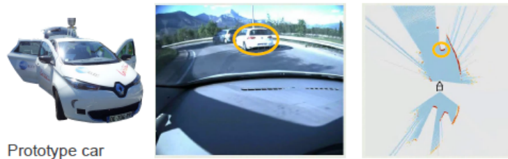
Figure 9. Fusion of three front LIDARs and one rear LIDAR on the ZOE platform
