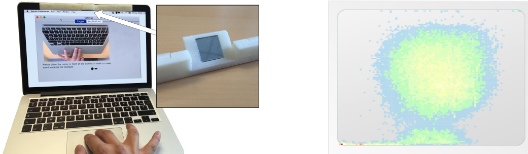
Figure 1. Left: Mirror positioned in front of a built-in camera to divert its field of view and analyze finger-chords usages; Right: frequency distribution of all touch events of our participants, overlaid on a trackpad.
