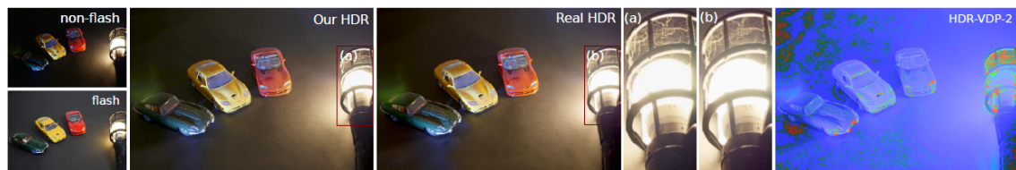
Figure 2. HDR image recovery from two input images, i.e. flash and non-flash images. Our HDR result and the real HDR image are tone-mapped for visualization on an LDR display.
