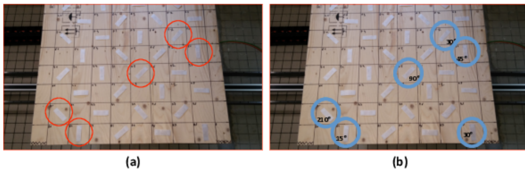
Figure 4. (a) initial read, 20% of the tags are missing (b) After 210 deg of rotation, all the tags are recovered
