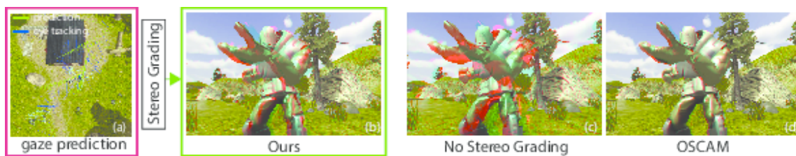
Figure 12. We propose a gaze predictor (a), used to perform localized stereo grading (b). We compare to no stereo grading (c) and prior work (d). We provide rich and comfortable depth. Please use red/cyan anaglyph glasses.
