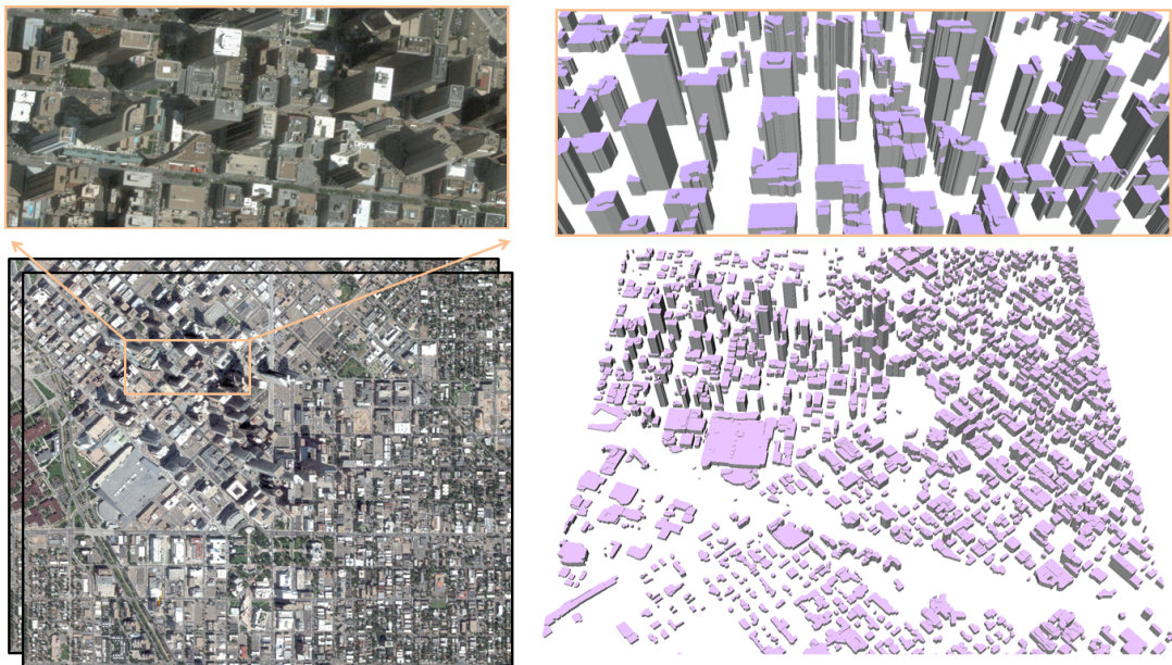
Figure 7. City reconstruction from satellites. Starting from a stereo pair of satellite images (left), our algorithm produces a compact and semantic-aware 3D model (right) in a few minutes.
