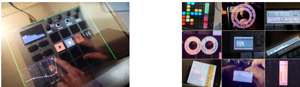
Figure 1. ControllAR: (left) ControllAR is used to augment a control surface with the remixed graphical user interface of music software, (right) Visual feedback designed by electronic musicians during our study belong to three categories: mappings feedback, processes feedback and content feedback.
