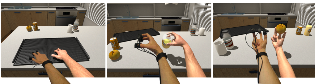
Figure 10. Illustrative use cases of our approach HapTip: the user can get in contact and tap a virtual bottle, touch a surface and feel its texture, and heft an object and feel its weight.
