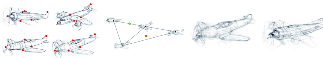
Figure 7. SketchSoup takes an unstructured set of sketches as input, along with a small number of correspondences (shown as red dots), registers the sketches and embeds them into a 2D interpolation space based on their shape differences. Users can explore the interpolation space to generate novel sketches.
