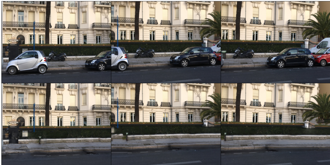
Figure 11. Our system takes as input a set of images from the same scene (top row). The method then removes all the vehicules in a multi-view coherent way (bottom row).
