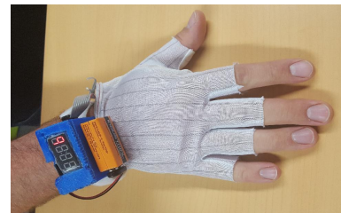
Figure 3. Instrumented glove for rehabilitation assessment
