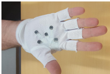
Figure 3. Instrumented glove for rehabilitation assessment
