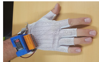
Figure 3. Instrumented glove for rehabilitation assessment
