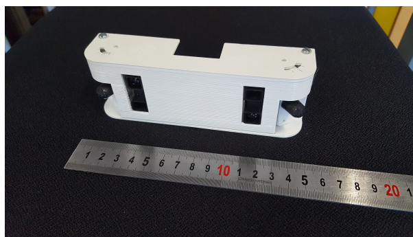
Figure 1. A station for activities detection. The 4 sensors allow to determine the presence of the subject in a given zone, his/her direction of motion and speed even at night
