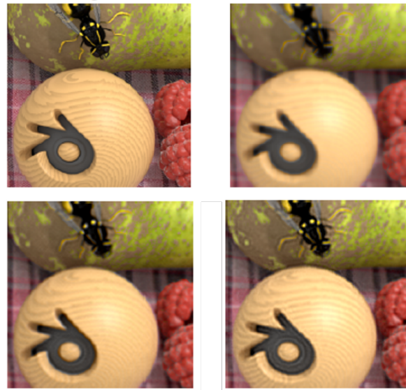
Figure 6. Illustration of some results on a crop of a central view with a magnification factor of 2; Top row: original (left), bicubic interpolation (right); Bottom row: super-resolved with a deep learning technique of the literature (left), super-resolved with the proposed method (right).
