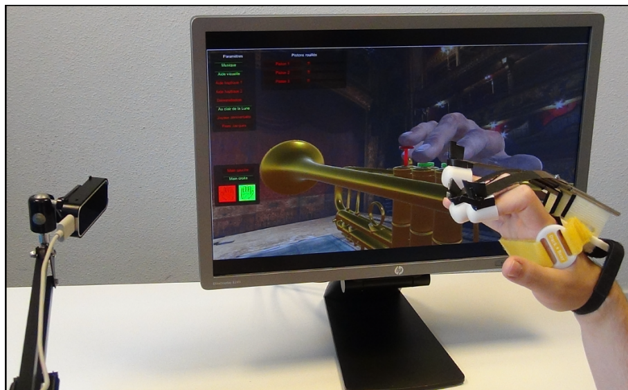
Figure 8. The FlexiFingers is a multi-finger device, combined with a pseudo-haptic approach, that can be used in music learning applications for instance.
