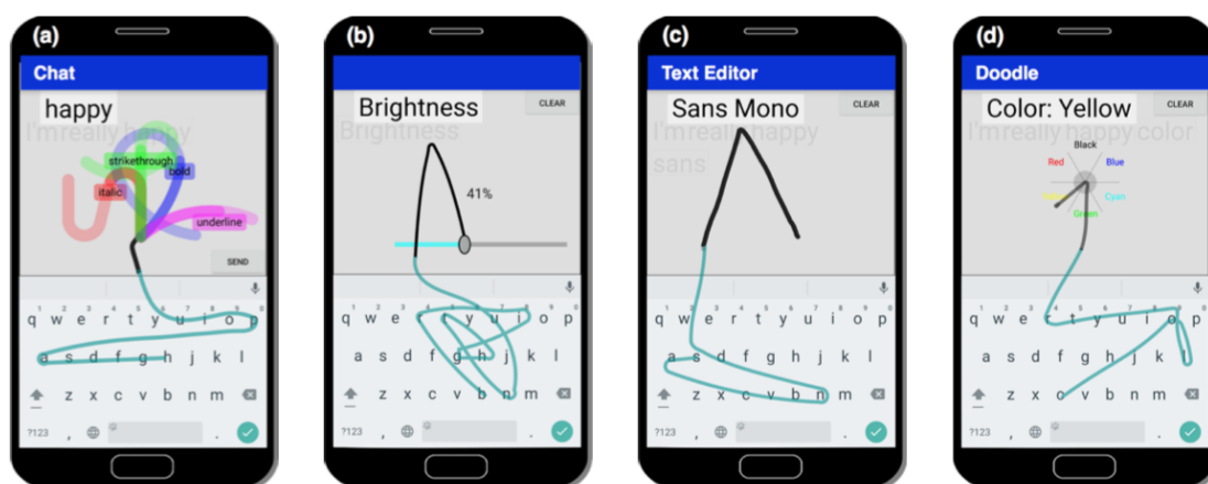
Figure 3. CommandBoard creates a new command gesture input space above a soft keyboard. Users can: a) type 'happy' and use a dynamic guide to style it as bold; b) type 'brightn', draw an execute gesture and adjust the brightness slider; c) type 'sans', choose 'sans mono' and draw an execute gesture to change the font; d) type 'color', select yellow in the marking menu to change the brush color.
