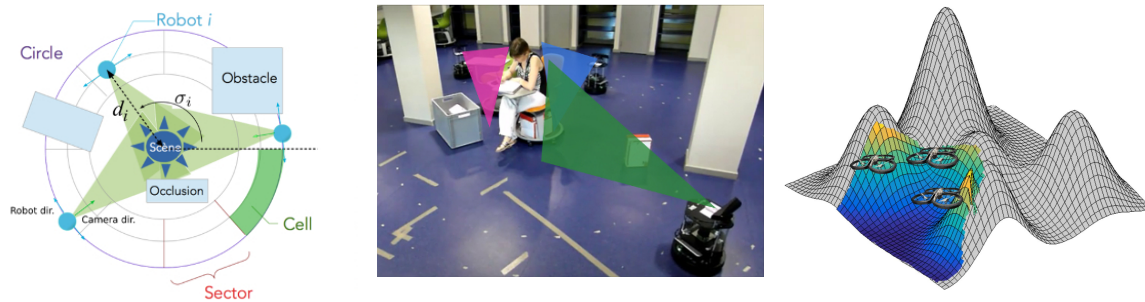
Figure 11. (a) Concentric navigation model and (b) its experimental setup. (c) Illustration of the local search method for multi-UAV coverage.
