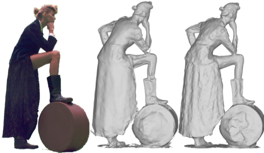
Figure 7. Challenging scene captured with Kinovis. (left) one input image, (center) reconstructions obtained with our previous work based on classical 2D features, (right) proposed solution. Our results validate the key improvement of a CNN-learned disparity to MVS for performance capture scenarios. Results particularly improve in noisy, very low contrast and low textured regions such as the arm, the leg or even the black skirt folds.
