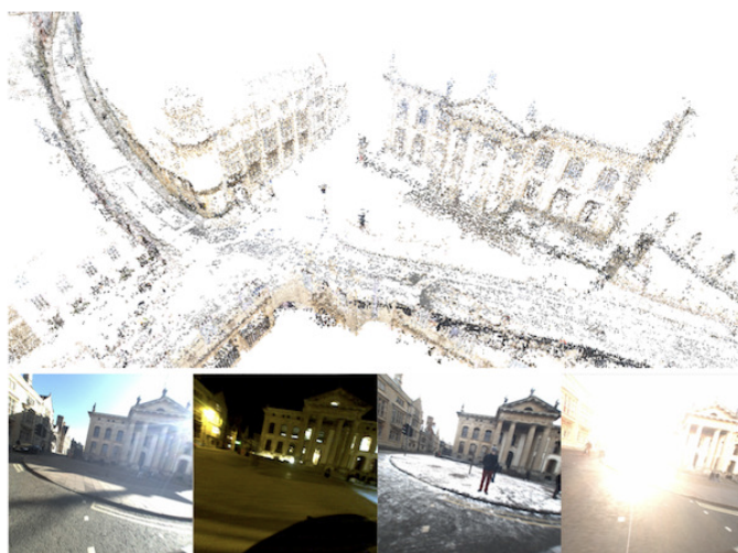
Figure 2. Visual localization in changing urban conditions. We present three new datasets, Aachen Day-Night, RobotCar Seasons (shown) and CMU Seasons for evaluating 6DOF localization against a prior 3D map (top) using registered query images taken from a wide variety of conditions (bottom), including day-night variation, weather, and seasonal changes over long periods of time.
