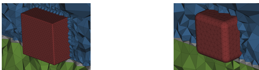
Figure 9. Meshes of rounded nanocubes with rounding radii ranging from 2 to 10 nm. Red cells correspond to the cube. The latter lies on the dielectric spacer (gray cells) and the metallic plate (green). Blue cells represent the air surrounding the device.
