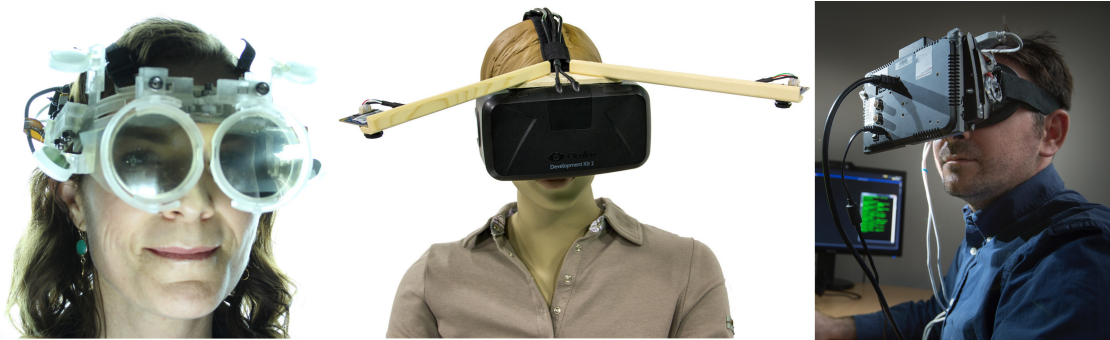
Figure 12. We presented novel display technologies, including but not limited to (left-to-right) varifocal augmented reality displays, body-tracking displays and focus-tunable displays.
