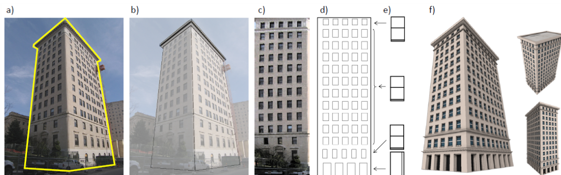
Figure 5. (a) Given an image and a silhouette of a building, (b) our approach automatically estimates the camera parameters and generates a building mass grammar as a first step. Then, (c) the facade image is rectified, and (d) the facade grammar is generated. (e) For each window non-terminal, the best window grammar is selected by maximum vote. (f) Finally the output grammar is constructed and a corresponding 3D geometry is generated.
