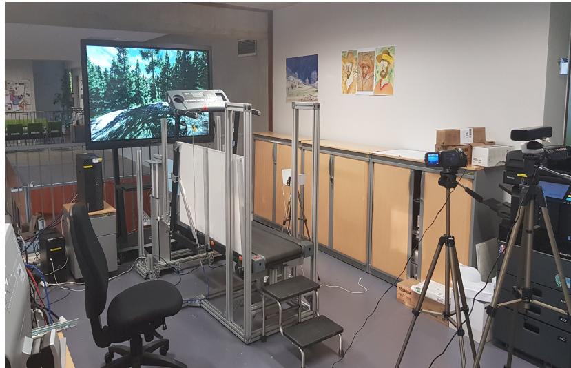
Figure 1. Our rehabilitation station in a configuration with a treadmill, 2 columns for changing its slope and inclination and lidar and kinect for motion analysis
