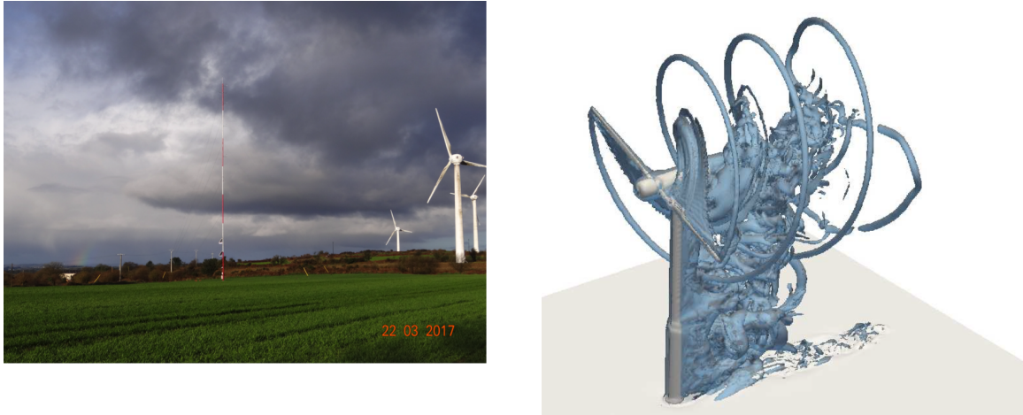
Figure 2. Aerogust project. Left: met mast after its installation. Right: flow around the optimized wind turbine rotor (as predicted by NaSCar).
