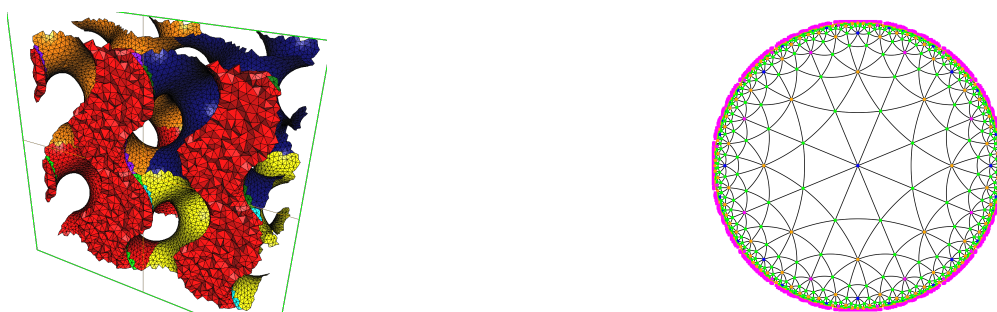
Figure 2. Left: 3D mesh of a gyroid (triplly periodic surface) [54]. Right: Simulation of a periodic Delaunay triangulation of the hyperbolic plane [24].
