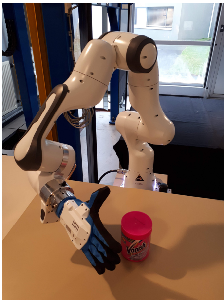
Figure 5. Rainbow advanced manipulation platform. One of the two Panda lightweight arms from Franka Emika, with mounted the Pisa SoftHand.
