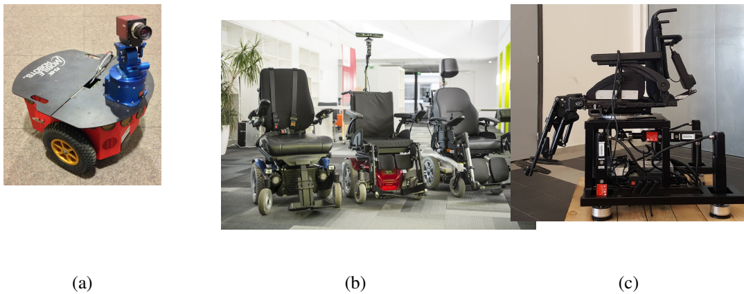
Figure 3. Mobile Robot Platform. a) Pioneer P3-DX robot, b) wheelchairs from Permobil, Sunrise and YouQ, c) the wheelchair haptic simulator.
