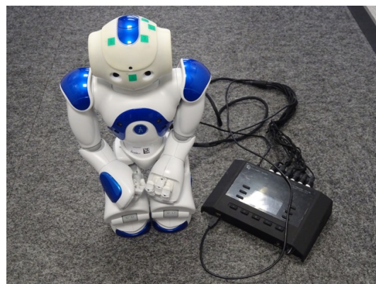
Figure 2. The Popeye+ audio-visual platform (left) delivers high-quality, high-resolution and wide-angle images at 30FPS. The NAO prototype used by PERCEPTION in the EARS STREP project has a twelve-channel spherical microphone array synchronized with a stereo camera pair.
