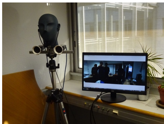
Figure 2. The Popeye+ audio-visual platform (left) delivers high-quality, high-resolution and wide-angle images at 30FPS. The NAO prototype used by PERCEPTION in the EARS STREP project has a twelve-channel spherical microphone array synchronized with a stereo camera pair.
