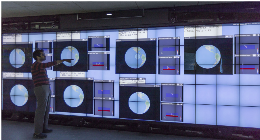
Figure 3. Multiple asteroid-generated tsunami simulations running simultaneously on the WILDER ultra-wall. The high display capacity of this interactive surface makes it possible to show, for each of the simulations: a planet-wide view showing the propagation of the tsunami on the globe, a close-up on the region of impact, showing a simulation of one or more scalar fields, parameters of the simulation.
