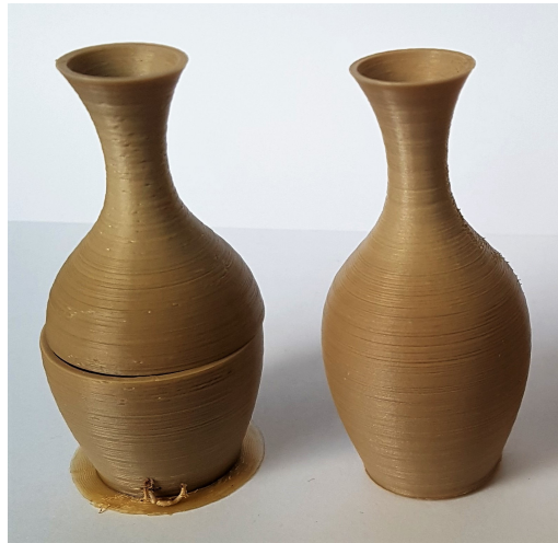
Figure 10. 3D printed vase in PEEK material. Left: Vase breaking during fabrication due to thermal stresses. Right: Adding a thermal shield (not shown) results in a correct 3D print.
