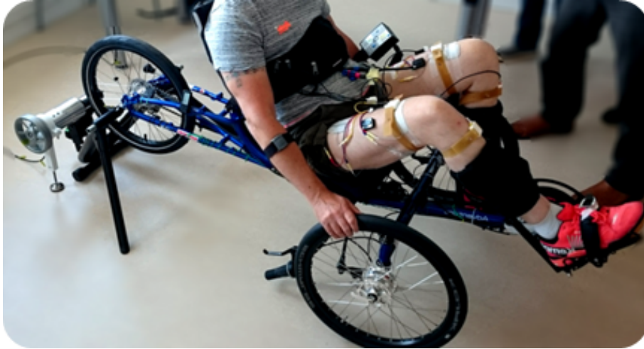
Figure 7. Experimental setup using IMUs to record joint angles and a specifically designed home trainer to monitor power output.
