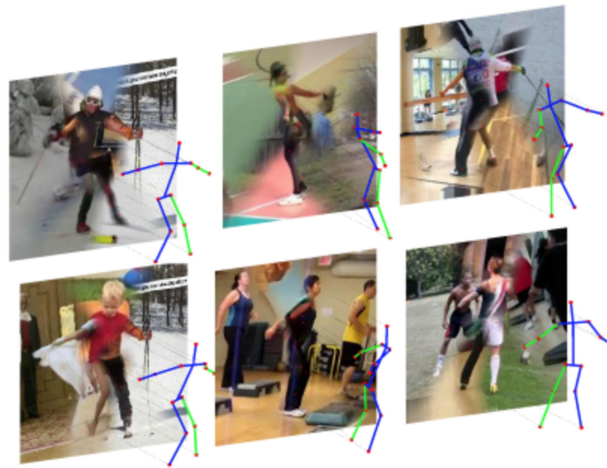
Figure 9. Given a candidate 3D pose, our algorithm selects for each joint an image whose annotated 2D pose locally matches the projected 3D pose. The selected images are then combined to generate a new synthetic image by stitching local image patches in a kinematically constrained manner. We show 6 examples corresponding to the same 3D pose observed from 6 different camera viewpoints.
