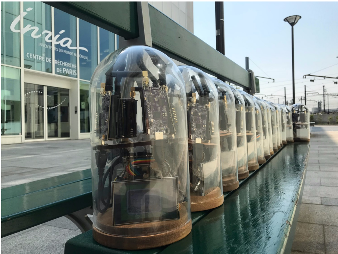
Figure 2. The OpenTestbed deployed in Inria Paris since July 2018.
