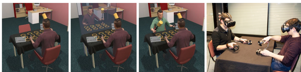
Figure 6. Setup of the experiment: each user was able to interact in the virtual environment with his own avatar, while the physical setup provided both a reference frame and passive haptic feedback. From left to right: experimental conditions Alone, Mirror and Shared; Physical setup of the experiment.
