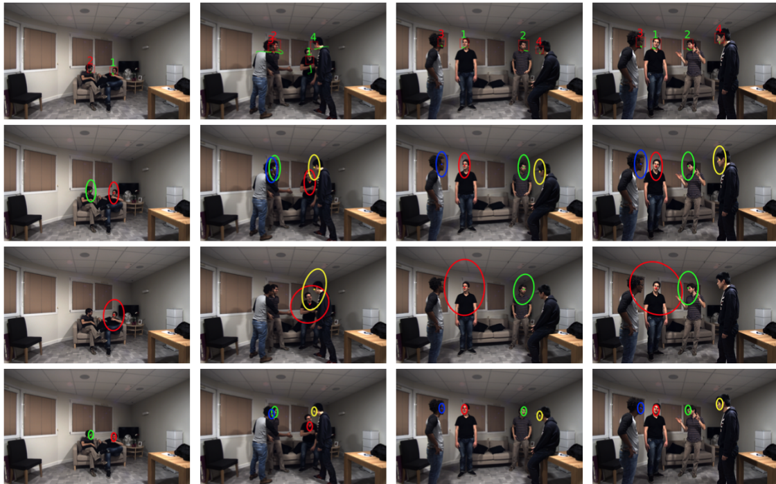
Figure 1. This figure illustrates the audio-visual multiple-person tracking that has been developed by the team [38], [41]. The tracker is based on variational inference [5] and on supervised sound-source localization [10], [29]. Each person is identified with a digit. Green digits denote active speakers while red digits denote silent persons. The next rows show the covariances (uncertainties) associated with the visual (second row), audio (third row) and dynamic (fourth row) contributions for tracking a varying number of persons. Notice the large uncertainty associated with audio and the small uncertainty associated with the dynamics of the tracker. In the light of this example, one may notice the complementary roles played by vision and audio: vision data are more accurate while audio data provide speaker information. These developments have been supported by the European Union via the FP7 STREP project “Embodied Audition for Robots” (EARS) and the ERC advanced grant “Vision and Hearing in Action” (VHIA).
