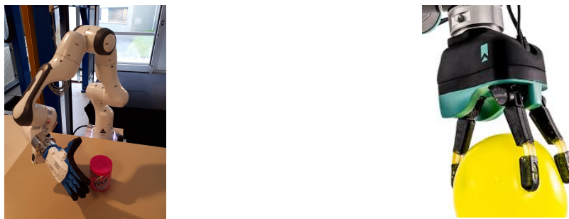
Figure 5. Rainbow advanced manipulation platform. a) One of the two Panda lightweight arms from Franka Emika, with mounted the Pisa SoftHand, b) the Reflex TakkTile 2 gripper that could be mounted on the Panda robot end-effector.
