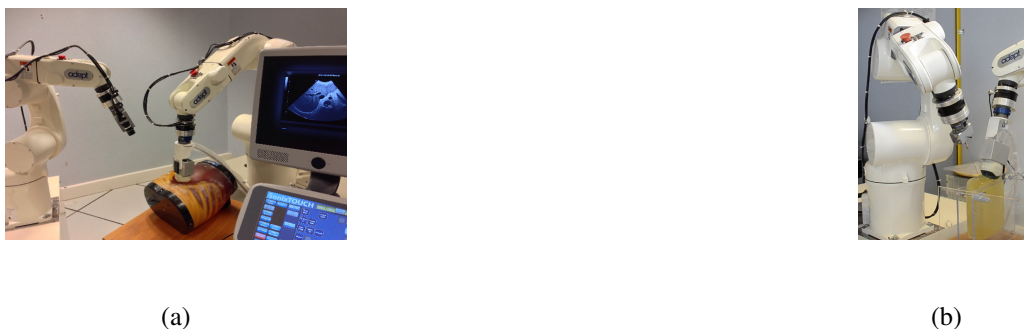
Figure 4. Rainbow medical robotic platforms. a) On the right Viper S850 robot arm equipped with a SonixTouch 3D ultrasound probe. On the left Viper S650 equipped with a tool changer that allows to attach a classical camera or biopsy needles. b) Robotic setup for autonomous needle insertion by visual servoing.
