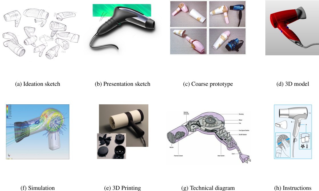
Figure 2. Various representations of a hair dryer at different stages of the design process. Image source, in order: c-maeng on deviantart.com , shauntur on deviantart.com , "Prototyping and Modelmaking for Product Design" Hallgrimsson, B., Laurence King Publishers, 2012, samshe511 on turbosquid.com , my.solidworks.com , weilung tseng on cargocollective.com , howstuffworks.com , u-manual.com
