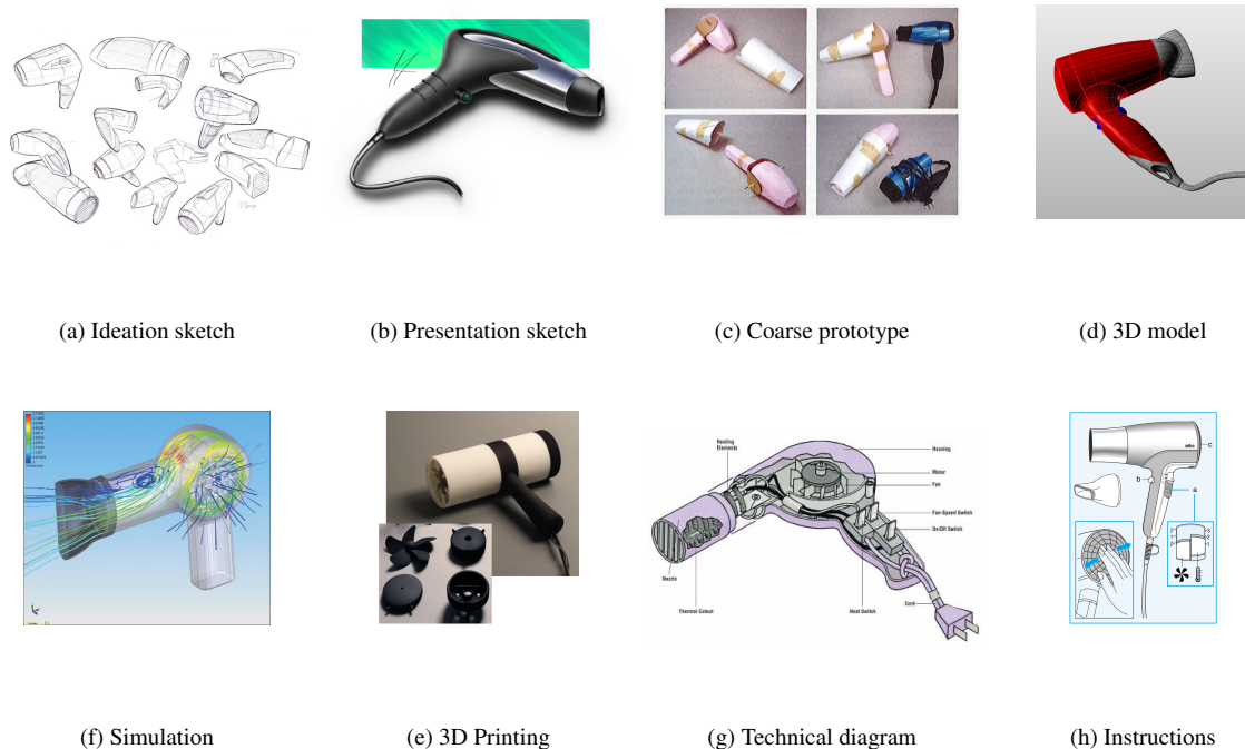
Figure 2. Various representations of a hair dryer at different stages of the design process. Image source, in order: c-maeng on deviantart.com, shauntur on deviantart.com, "Prototyping and Modelmaking for Product Design" Hallgrimsson, B., Laurence King Publishers, 2012, samsher511 on turbosquid.com, my.solidworks.com, weilung tseng on cargocollective.com, howstuffworks.com, u-manual.com
