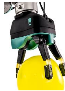
Figure 5. Rainbow advanced manipulation platform. a) One of the two Panda lightweight arms from Franka Emika, with mounted the Pisa SoftHand, b) the Reflex TakkTile 2 gripper that could be mounted on the Panda robot end-effector.
