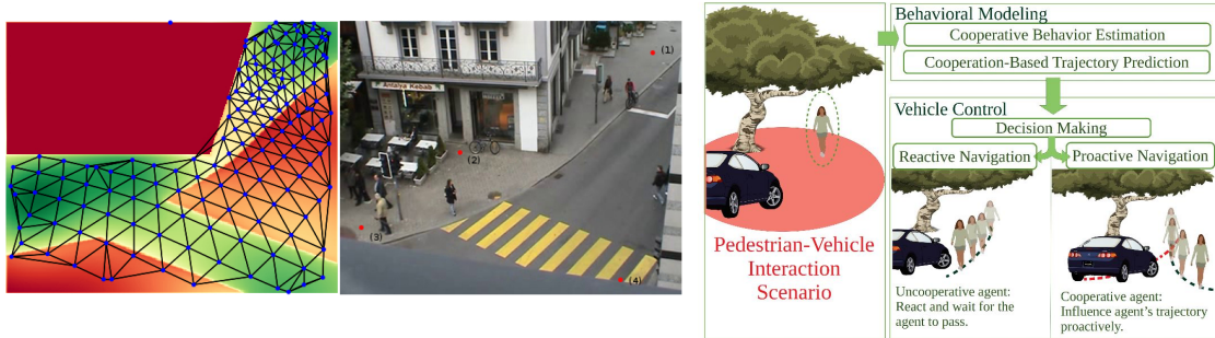
Figure 17. a. Prior Topological Map of the dataset from the Traffic Anomaly Dataset : first figure shows the generated potential cost map and second figure the “Prior Topology” of the image from scene. b. Illustration of the Principle of Proactive Navigation.
