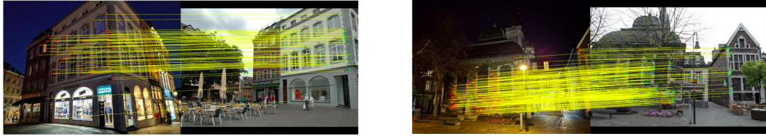
Figure 9. The scene coordinate predictions are visualized as 2D-2D matches between the query (left) and database (right) images. For each pair, the retrieved database image with the largest number of inliers is selected, and only the inlier matches are visualized. We show that our method is able to produce accurate correspondences for challenging queries.
