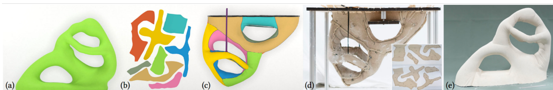
Figure 2. A fertility model designed and fabricated using our computational approach. For a target 3D model (a), our system can automatically compute a set of flat panels (b) that can be sewn together to serve as fabric containers to form a target shape by pressure of liquid plaster poured in – see (c) for the simulation under force equilibrium of membrane tension, liquid pressure and external supports. The generated flat panels are used to conduct the physical fabrication of fabric formwork (d). After drying and unwrapping the fabric container, a sculpture with the designed target shape has been fabricated (e).
