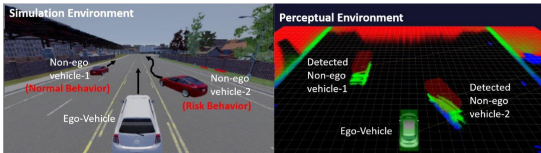
Figure 14. (Left) Simulation environment with CARLA simulator. The white vehicle is the ego-vehicle and two non-ego vehicles are simulated to perform anomaly movements. (Right) Perceptual environment with CMCDOT framework. By analyzing the real-time velocity and position of vehicles, the state and behavior of vehicles can be inferred.
