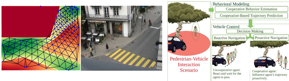
Figure 17. a. Prior Topological Map of the dataset from the Traffic Anomaly Dataset : first figure shows the generated potential cost map and second figure the “Prior Topology” of the image from scene. b. Illustration of the Principle of Proactive Navigation.
