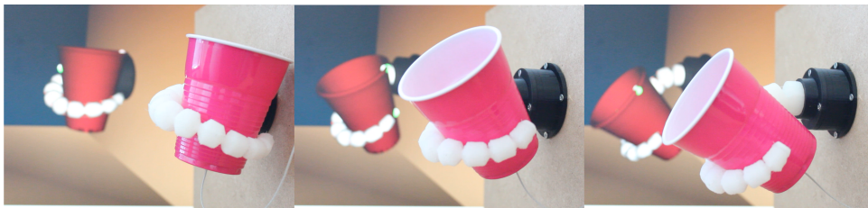
Figure 3. Real soft robot actuated online using the output of the simulation. In this scenario, using our control framework, we are able to control the orientation of the real plastic cup (see the attached video).
